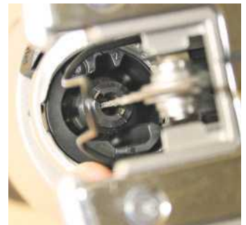
▲ Once fitted the collar wraps around the shank to lock it in place
